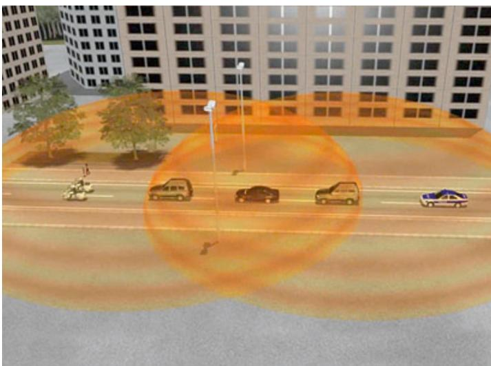
Two jammer vehicles establish protective perimeter around VIP vehicle.
